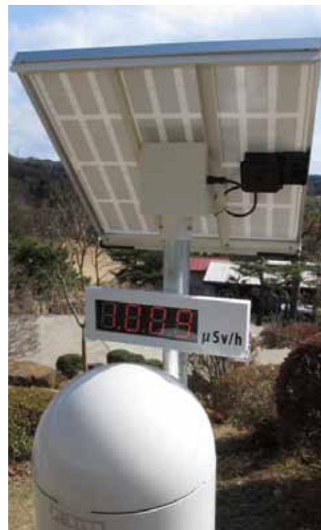
The Japanese government installed solar powered dosimeters at every school and children’s home in Fukushima. The radiation level during our visit in March was 1.009μSv/h, which is the highest constant level of any children’s home in Fukushima Prefecture (a normal level would be 0.009μSv/h).
